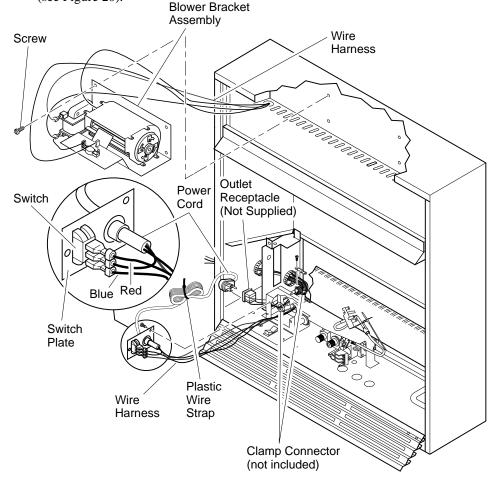
Figure 19 - Installing Blower Bracket Assembly
